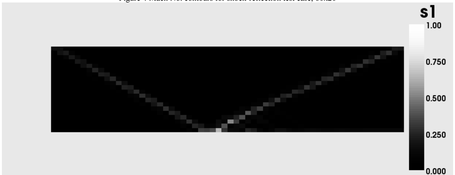
Figure 5 The first order implicitness parameter s_1 contours for shock-reflection test case, 60x20
