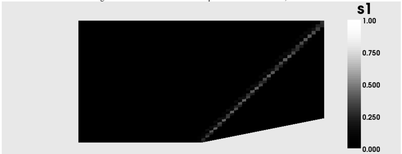
Figure 10 The first order implicitness parameter s_1 contours for compression-corner test case, 60x40
